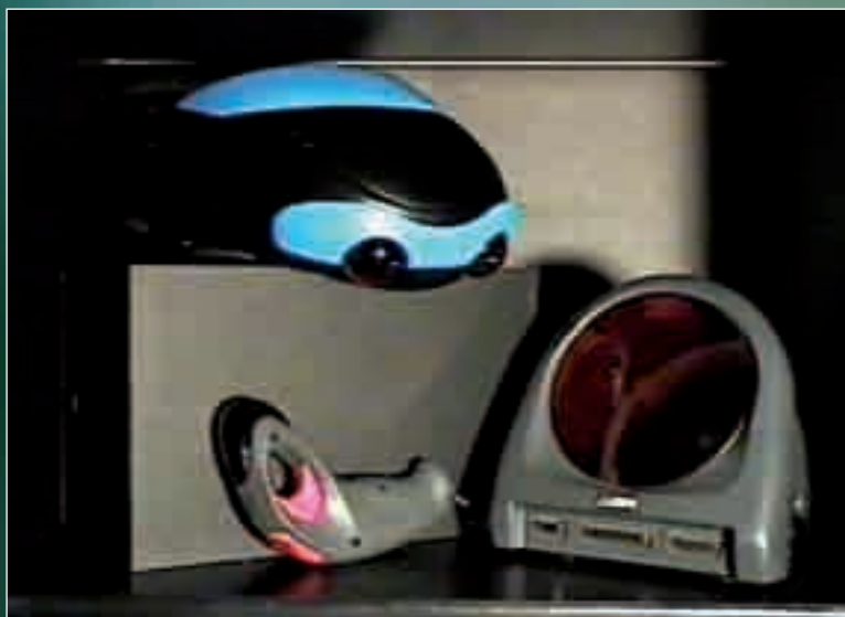
» Jaguar VR prototype unit – note the motion tracking spheres on the headset.
